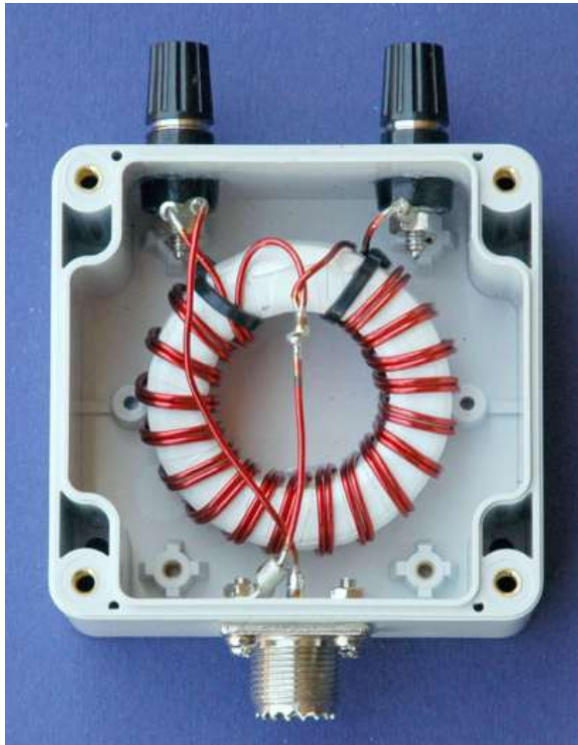
Photo 1 4:1 Ruthroff voltage balun assembled.
