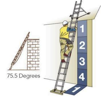
It might be tempting to just pop a ladder up and climb up to fix or adjust something, this is the way that accidents can happen. Remember to take that little bit of extra time to ensure that your ladder is secure: the base can't slip away, the top is resting against a secure spot. Some ladders come with or can have added to them, additional ties, straps or extensions that can make the ladder more secure. If you have these desirable features please use them.
