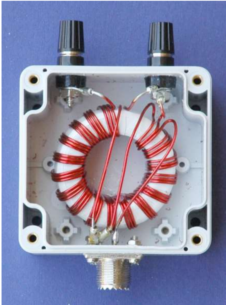
Photo 1 1:1 Ruthroff voltage balun assembled.
