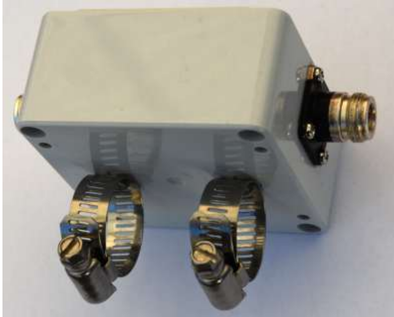
Photo 2 Rear view of the Low band choking balun assembled showing the hose clamp mast attachments.
