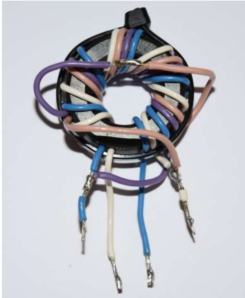
Photo 1 1:6 Voltage balun assembled.
