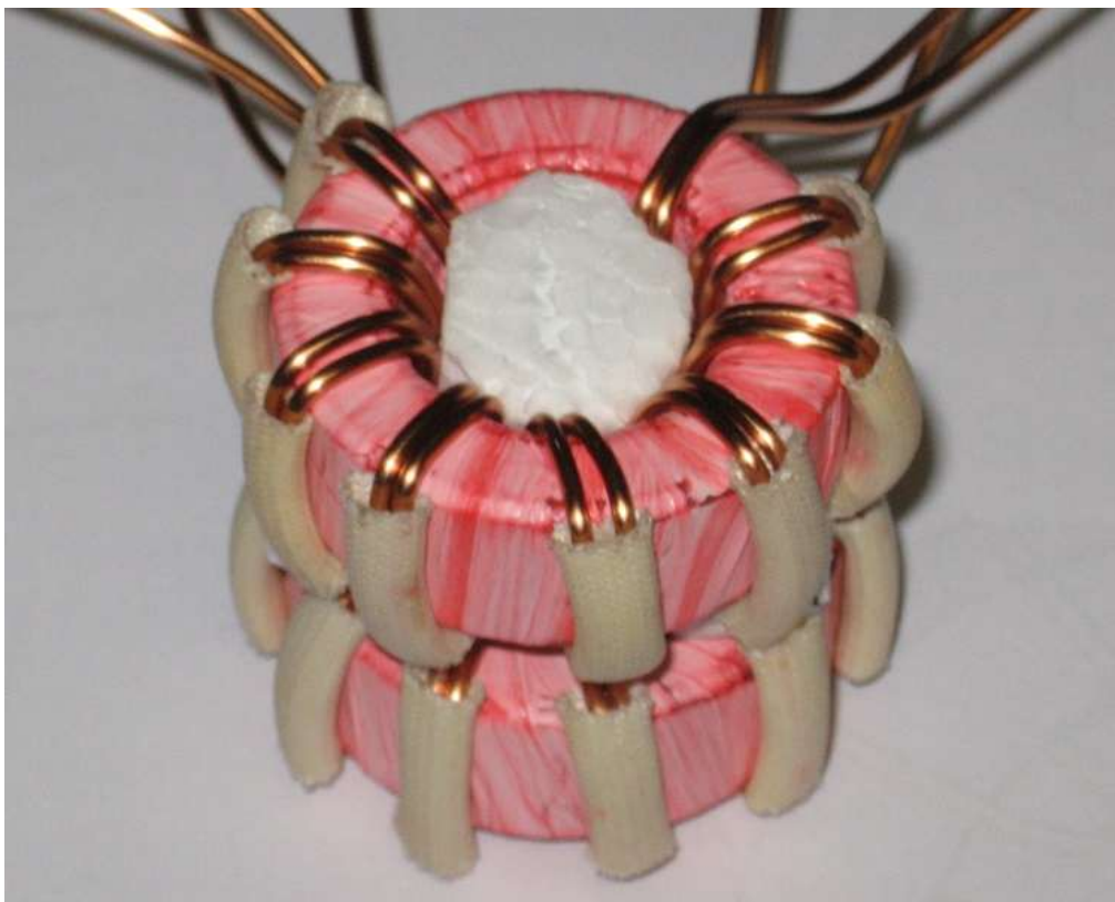
Photo 2 1:4 Guanella current balun individual core windings stack assembled.
