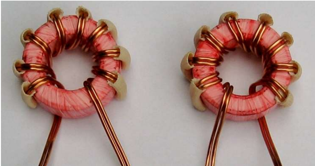
Photo 1 1:4 Guanella current balun individual core windings assembled.
